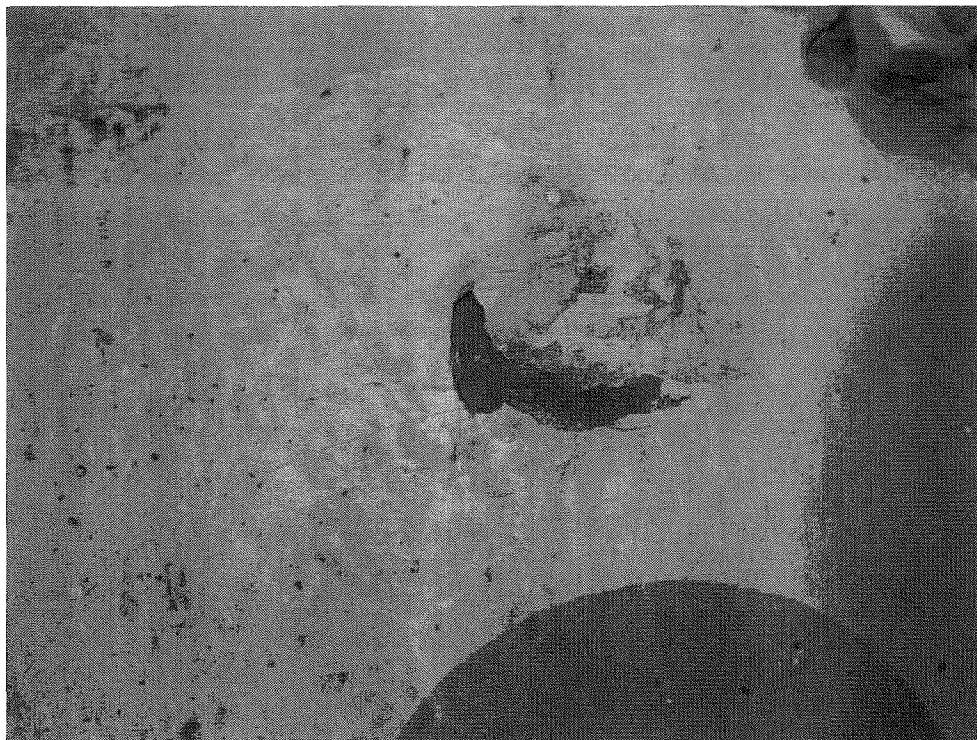
Figure 13 - Photograph showing the area of Valve 3 that was selected to be polished and have Replicas made.
