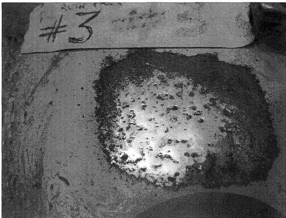
Figure 14 - Photograph of the area on Valve 3 shown in Figure 5 after polishing
