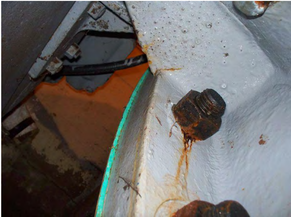
Crack through coating in area opposite flange (from area above in photo 3291)
