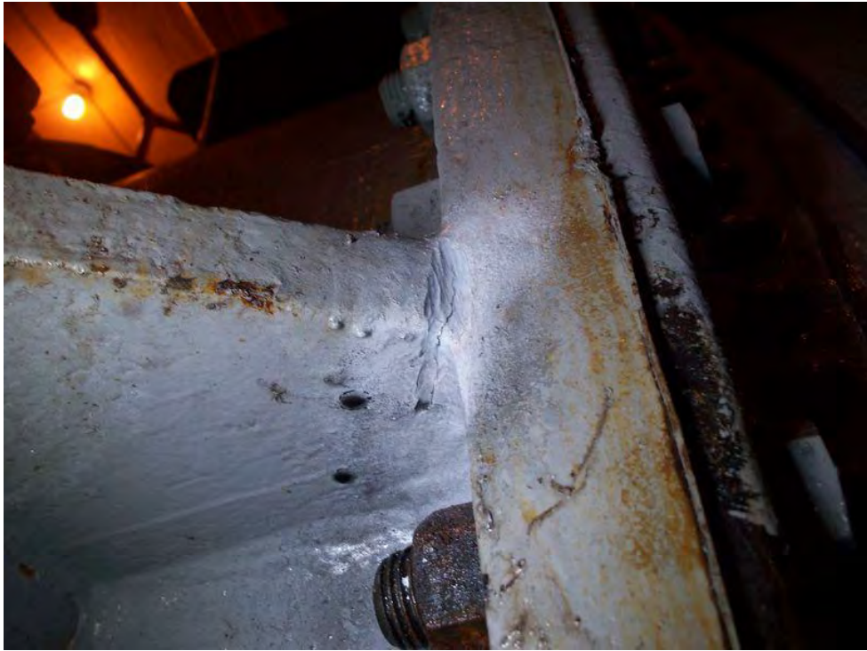
Close-up of crack (MPI) indication in area of photo 3289
