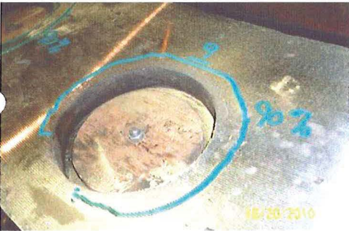
HOLE #9 WITH LINEAR INDICATION 90% AROUND HOLE
