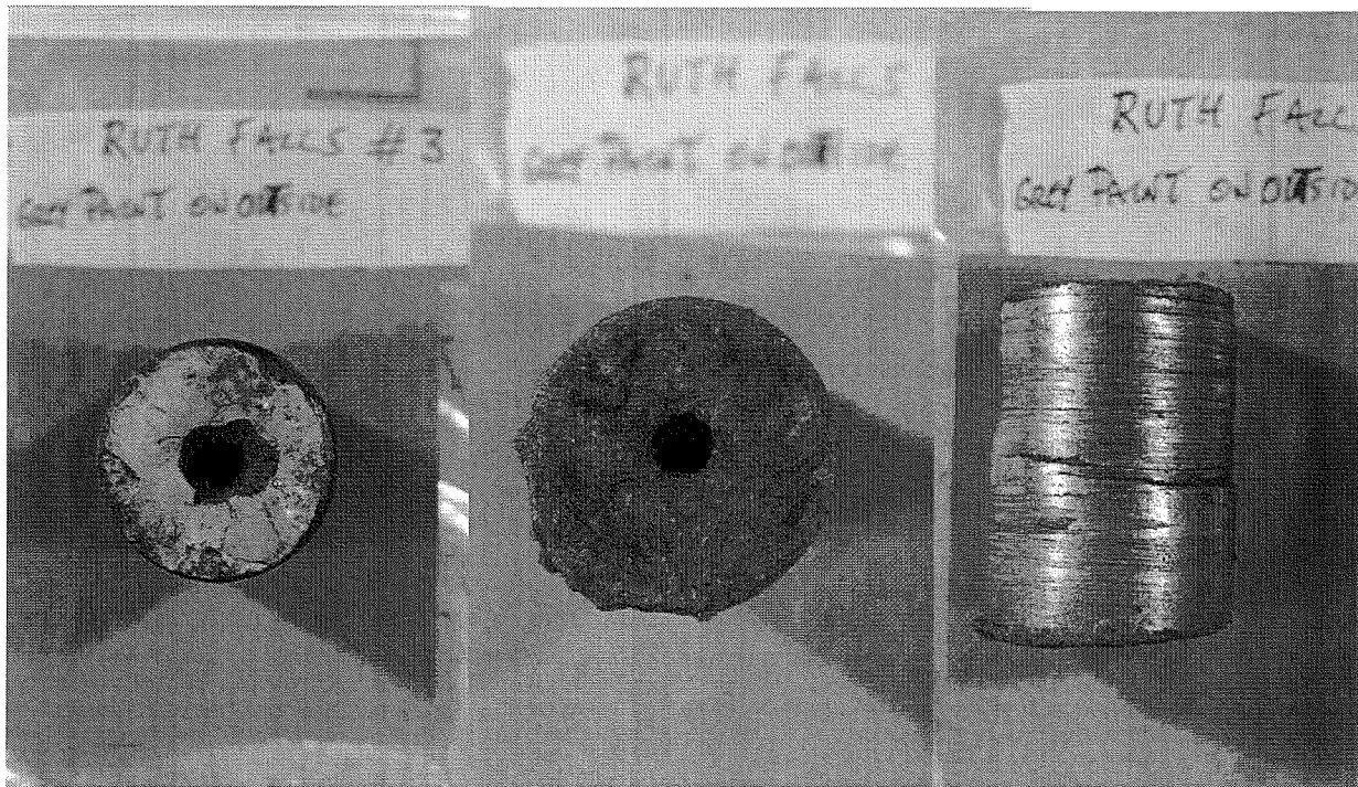
Figure 16 - Photographs showing the painted side, scale side, and profile of the core sample taken from Valve 3
