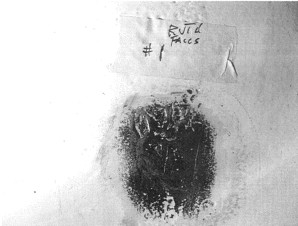
Figure 7 - Photograph of the area of Valve 1 shown in Figure 3 after polishing
