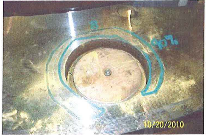
HOLE #8 WITH LINEAR INDICATION 90% AROUND HOLE
