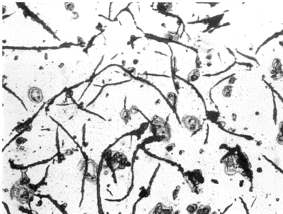
Figure 17 Micrograph of the Core Sample from Ruth Falls #3 Valve Butterfly. 100X
